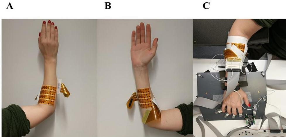
Fig. 1. Experimental setup. (A) Placement of HD-EMG grid on extensor, and (B) flexor muscles of the lower arm. (C) Custom made force device.
